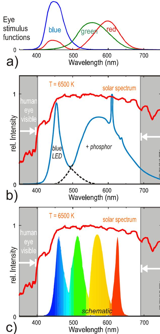
**Figure 1** a) Human eye response curves revealing three rather distinct channels of sensitivity. b) The midday solar spectrum on earth and current white light LEDs utilizing a narrowband blue source and broadband yellow phosphors. In advanced designs a narrow band red phosphor is added. c) A schematic of combining blue, green, yellow and red LEDs to provide a more even approximation of the solar spectrum for enhanced color fidelity.
