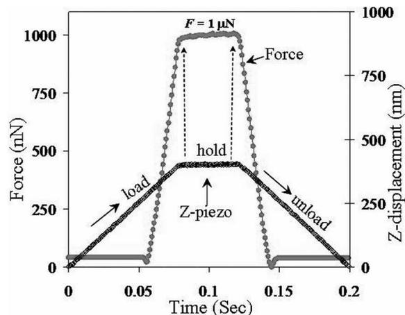
FIG. 2. Time variation of the applied force and the Z-displacement signals from the AFM during a loading-unloading cycle. The force is limited to a specified value (here  $1 \mu\text{N}$ ) and is held at the upper limit for a short duration.
