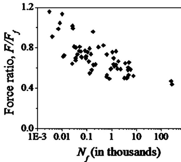
FIG. 6. The variation of fatigue life (number of cycles to failure) with the applied maximum force,  $F$ . The amplitude and the mean of the cycle are both equal to  $F/2$ . The vertical axis is normalized by the monotonic failure force,  $F_f$  (Fig. 3).
