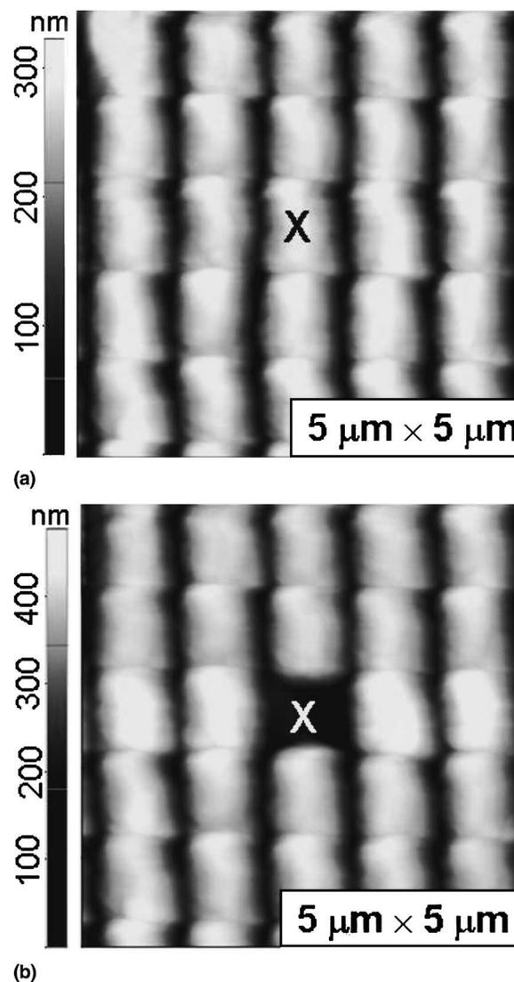
FIG. 5. Topographic AFM images of the sample area (a) before and (b) after the cyclic test. The specimen marked by “X” in (a) is loaded and fails, so is not present in (b).
