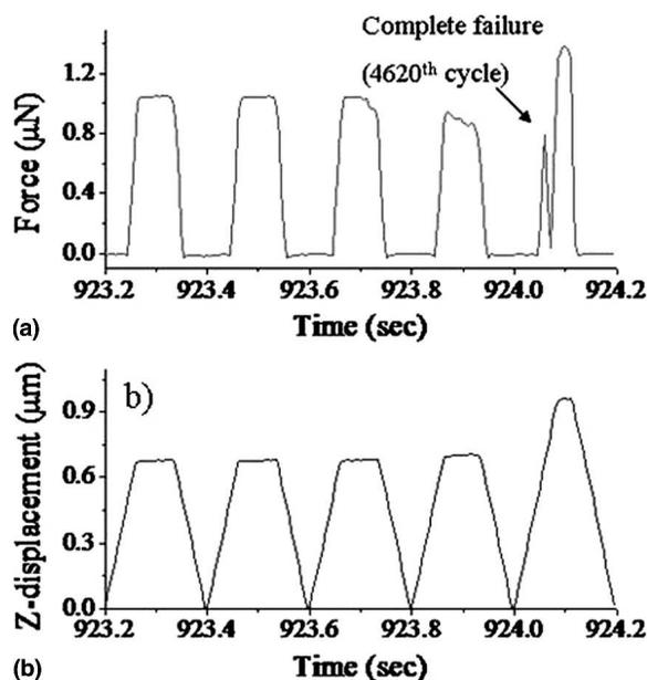
FIG. 4. (a) Force waveform and (b) the accompanying Z-displacement plotted against time showing the failure of the specimen. In this particular test, a peak force of 1050 nN was used and the failure resulted in the 4620th cycle as indicated by the instability in force as well as Z-displacement waveforms. The first of the two peaks in the last cycle corresponds to the response from the specimen, the dip corresponds to failure, while the second peak is due to the cantilever loading the substrate.
