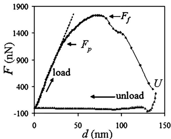
FIG. 3. A typical  $F-d$  curve obtained in a monotonic loading test.  $F_p$  and  $F_f$  indicate the limit of proportionality and the failure force, respectively. Beyond  $F_f$ , the specimen fails and the force decreases; however, unloading (retraction of the tip) begins at U.
