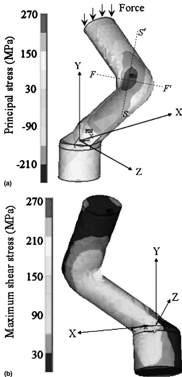
FIG. 9. (a) Maximum principal and (b) maximum shear stress distributions obtained by finite element modeling and corresponding to an applied force of 1000 nN. The dotted line  $SS'$  represents the direction in which the maximum tensile principal stress acts, while the dotted line  $FF'$  shows the approximate failure plane observed in experiments. Note that both stresses are highest at the turning point of the elbow [A in Fig. 1(a)].
