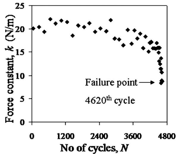
FIG. 7. The variation of the measured specimen stiffness,  $k$ , during cyclic loading. Initially the stiffness was evaluated every 200th cycle, after  $\sim 0.7N_f$  every 50th cycle, and after  $\sim 0.9N_f$  every 10th cycle. The stiffness is approximately constant up to  $\sim 0.8N_f$ , while in the final  $\sim 0.2N_f$  cycles it decreases abruptly.
