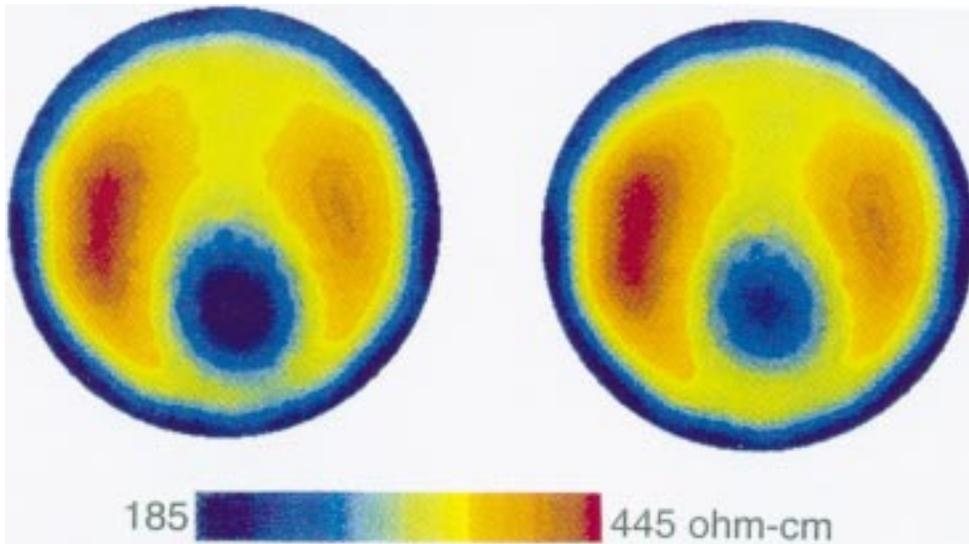
**Fig. 2** Images of the resistivity of two different test tanks like the one shown in Figure 1. The two different tanks had hearts of different sizes, meant to simulate different times during the heart’s cycle.
