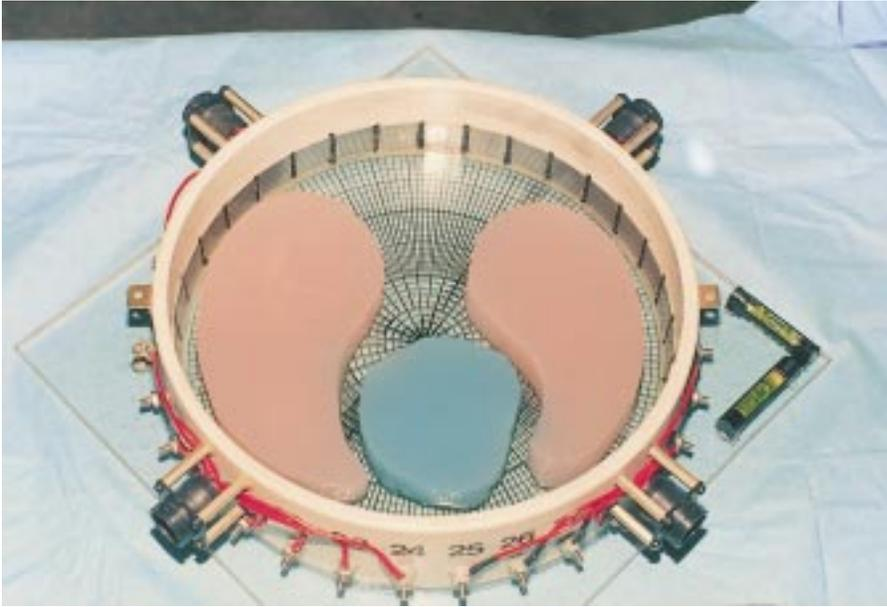
**Fig. 1** A test tank containing “lungs” and “heart” made of agar with varying amounts of added salt. This tank is filled with salt water, and used as a test body for the EIT system. Note the large electrodes around the inner circumference of the tank.
