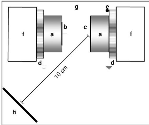
FIG. 1. Setup for paired-crystal neutron generation experiments. (a) 20 mm dia.  $\times$  10 mm thick  $\text{LiTaO}_3$  crystal. (b) 3 mm long catwhisker tip with  $0.07 \mu\text{m}$  apex mounted to a 13 mm dia.  $\times$  1 mm thick Cu disk. (c) Deuterated polystyrene target. (d) Thermoelectric heater/cooler. (e) Thermocouple. (f) Cu heat sink. (g) Vacuum chamber filled with 1.2 mTorr  $\text{D}_2$  gas. (h)  $3'' \times 3''$  EJ-301 detector at  $45^\circ$  angle to crystals.
